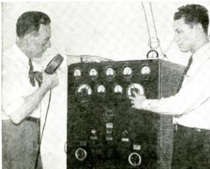
Experimental 8-meter transmitter used in demonstrating the value of ultra short-waves before the Newark, N. J., Police Dept. Paul F. Godley appears at the left with the "mike," while the engineer at the right of the photo is Edmund La Port.
